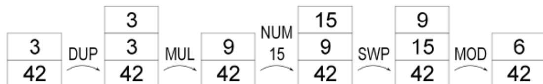
All binary operations consider the top-most number to be the “right” operand, the second number the “left” one. All of them remove both operands from the stack and place the result on top in place of the original numbers.
