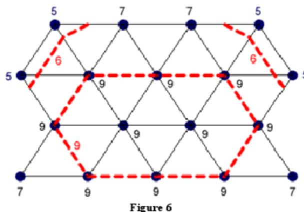
The policy of the ACM is to approximate the actual terrain by a set of triangles constructed by connecting each elevation measurement to its nearest neighbors by straight line segments. Each of these triangles is then treated as a planar surface, where the plane is determined by the coordinates, including elevation, of the vertices. If the triangles are projected onto the zero-elevation plane, they form a set of equilateral triangles.
