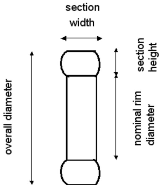
The *overall circumference* (the goal of your calculations) is based on the *overall diameter*, which is the diameter of an inflated tire at the outermost surface of the tread.
