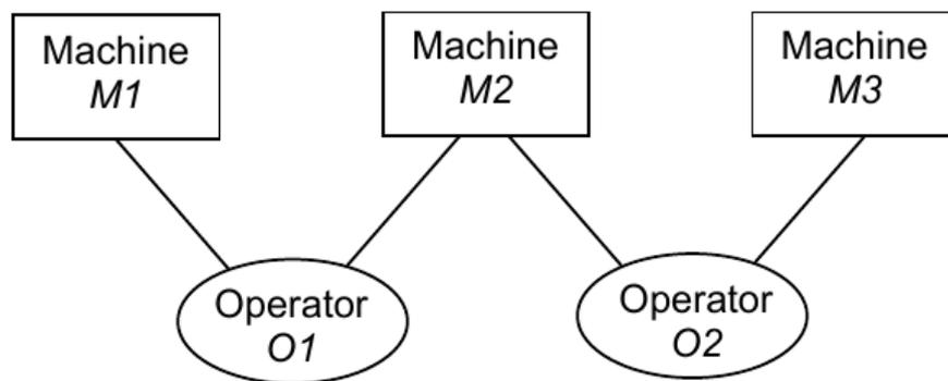
Machines and operators are modeled as resources in simulation. The relationship between machines and operators can be defined as follows: machine  $X$  and operator  $Y$  are related to each other (written as  $X \leftrightarrow Y$ ) if  $X$  and  $Y$  are required in the same processing step. Note that relation  $\leftrightarrow$  is symmetric. An equivalence class can then be defined by the transitive closure of this relation (written as  $\leftrightarrow^+$ ). For resources  $X$  and  $Y$ ,
